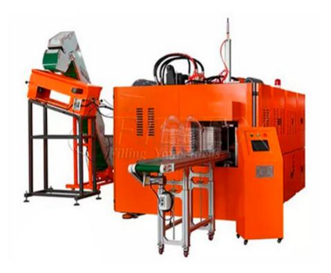
Full automatic blow molding machine is suitable for producing PET plastic containers and bottles in all shapes. It is widely used to produce the carbonated bottle, mineral water, pesticide bottle oil bottle cosmetics, wide-mouth bottle and hot fill bottle etc.
