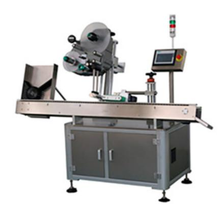
This labeler is designed for cylindrical body or bottles with small diameter. It cannot stand alone and be conveyed steadily. Such as injecting bottles, dry cells, pens, and so no.
