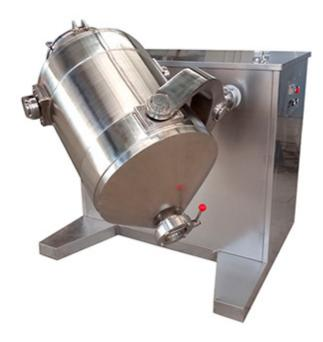
The mixing cylinder of this machine moves in many directions, the material has no centrifugal force, no specific gravity segregation and layering, accumulation phenomenon, each component can have a disparate weight ratio, the mixing rate is more than 100%, it is the most ideal product in various mixers at present .
