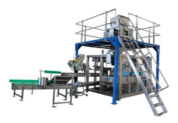
SGJ-ZD Automatic Bagging Packaging Machine Unit Is An Machine Which Can Be Used For Packing 10 - 50KG Material Into Big Sack Or Woven Bag. The Bagging Machine Unit Adopts Automatic Bag Feeding Device Which Can Feed Bag Automatically. And For The Material Weighing, Filling, Bag Conveying, Bag Mouth Folding And Sewing Shall All Accomplished By This Bagging Machine Automatically.
