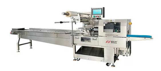
Flow Wrapping, or Horizontal Form-Fill and Seal (HFFS) is the process of making a horizontal bag from a single roll of film. Heat is applied to the bottom and ends of the film to form a sealed, flexible package already filled with products. Flow wrap packaging is used for a variety of products from food and baked goods to regular household items and stationary.
