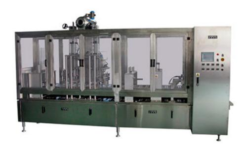
Horizontal Plastic Cup Fill & Seal Machine is suitable for liquid and paste such as pure milk, acidophilus milk, milk beverage, soybean milk, juice, ice cream, seasoning, daily chemical and etc. And also suitable for soft granule in the size of less than 8mm.
