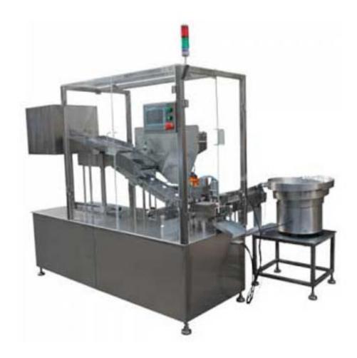
PZG-40 Effervescent Tablet Packaging Machine is designed for pharmaceutical, foodstuff, chemical etc. manufacturing and is based on a well-proven technology for rapid and gentle filling of tablets in rigid tubes. PZG-40 Effervescent Tablet Packaging Machine is fully GMP conform and can deliver a nominal capacity of 30 tubes/min.
