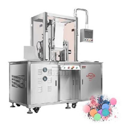
JBC-3 Bottom up Powder Compact Machine is suitable for cosmetic powders, such as face powder, blusher and eyeshadow. It can be used for handling a wide range of formulations. The machine can press embossed, engraved cakes and domes. The output is 720-1080 pcs/hour depending on pan size and powder formula.
