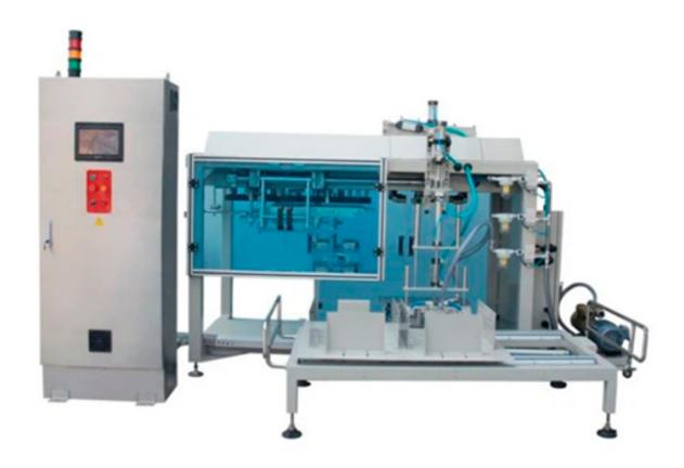
The whole machine is consisted of bag storage platform, bag taking mechanism, bag opening mechanism, sleeving mechanism, bag shaking mechanism, bag holding mechanism, machine frame and control box.
