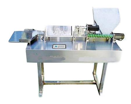
SYD semi-automatic lamp Inspection Machine is the second artificial light to achieve further development of the invention of semi-automatic control in mechatronic servo motor. Inspection light moving from the half-plane transmission reverse integration, through the organic visual black and white double-sided magnifying glass, the unqualified Automatic tick bottles of mechanization drive.
