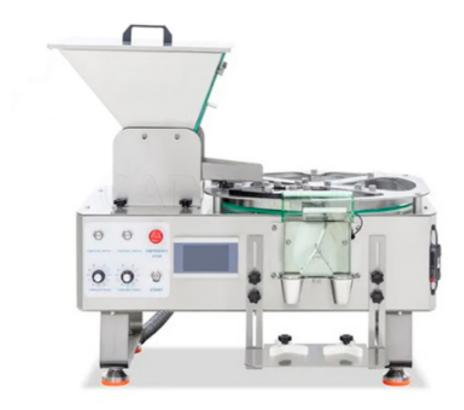
YL-2B semi-automatic counting machine is designed for efficient and accurate counting of various granular materials such as capsules, tablets and pills. It adopts the principle of photoelectric induction, and realizes continuous counting of single particles through vibration feeding and rotary centrifugal discharge, which is suitable for pharmaceutical, food and other industries.
