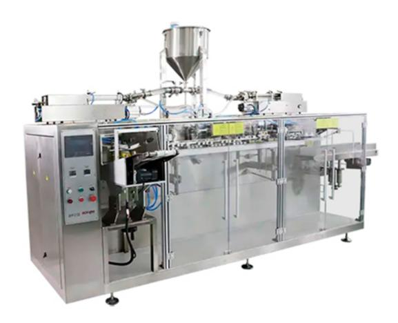
BHP-280D is specially designed for large bags. It has two sets of workstations and can package and produce two bags at the same time, doubling the production capacity. The packaged bag sizes are diverse, making it more convenient to change bag sizes. It can package a wide variety of materials and is suitable for wide range to meet most of the needs of customers.
