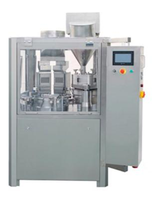
It is an intermittent full automatic capsule filling machine with multiple tamping stations, precise design and stable performance.
