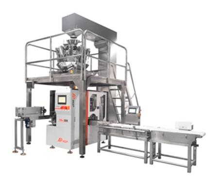
The FM200 bag packaging machine has good stability, high control accuracy, and does not come into contact with the packaging materials, which not only ensures the cleanliness of the packaging materials but also extends the service life of the machine. It uses multi-station rotary packaging, which effectively saves time and improves packaging efficiency.
