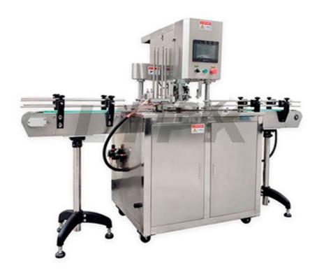
Can sealing machine is designed to automatically place lids onto cans and then seal them to ensure the contents remain airtight and protected from contaminants. This machinery plays a crucial role in food, beverage and other industries where products are stored in cans.
