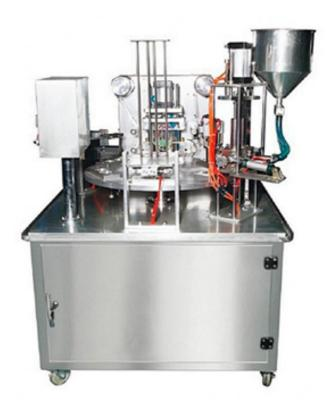
KIS-900 rotary type plastic cup filling and sealing machine suit for packing different density of beverage and paste products, as jelly, milk, ice scream, tallow, jam, juice and so on. this machine can be used for packing and sealing with various relevant composite film. This machine is widely used for different shape and volume containers (cups), and we can customize the machine as different request from customers.
