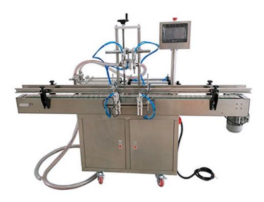
This machine is widely used filling liquid, semifluid liquid, such as liquid soap, shampoo, oil, and so on.
