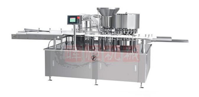
It's just for 10-20ML oral filling&sealing, a major machine in production line for oral liquid, it main used in filling, capping placing and sealing of straight tube bottle. Tracking filling, cap automatically conveying by electromagnetic oscillator, three knifes centrifugal sealing (or screwing), no bottle no filling. Filling and sealing integrated in one machine, advanced design, compact structure and completely comply with requirement of GMP.this kind of machine.
