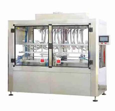
This machine is a high-tech filling equipment controlled by PLC, imported photoelectric sensor and imported pneumatic actuator. It can automatically complete a series of operations such as incoming bottle counting, servo motor driven quantitative filling and outgoing bottle conveying. This machine is an ideal packaging machinery and equipment specially designed for daily chemical, pharmaceutical, cosmetic and food industries.
