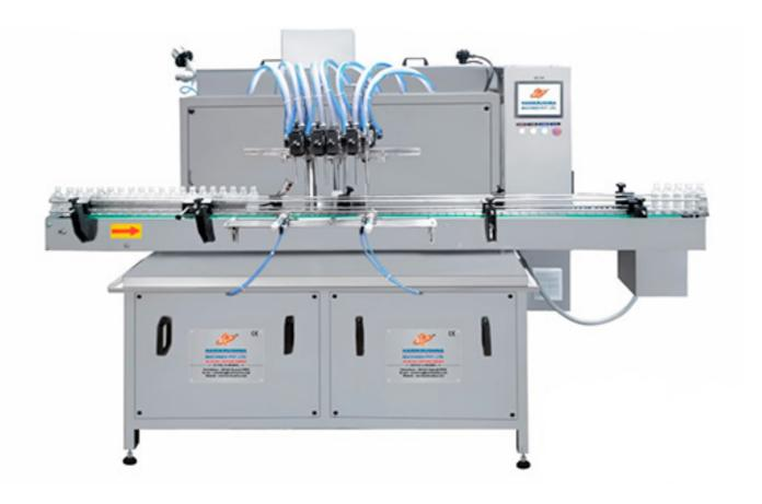
The Automatic Servo Liquid Filling Machine consists of a main structure, product transmission belt with an adjustable guide, material storage tank, pneumatic bottle stopping facility, SERVO-based Servo Liquid filling pumps, Servo Liquid filling nozzles, safety polycarbonate enclosure (OPTIONAL), electrical panel, motor, PLC & HMI, AC drive. A High / Low liquid level sensor in the tank is an added advantage.
