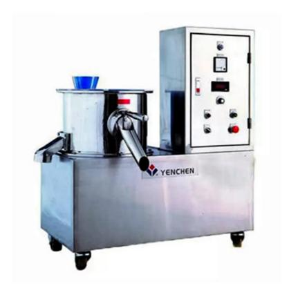
Pelletizer machine is suitable for producing round or ball shape granule. The process is to rolling long granule into required round pellet or balls.
