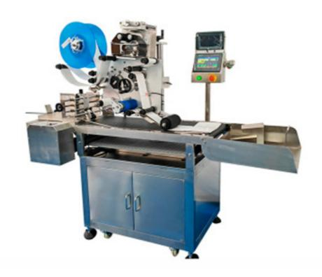
This series is widely used in the automatic labeling of clothing tags, cards, telephone cards, paper cards, and other objects; it has the functions of paging positioning and automatic labeling. This model can improve production efficiency and reduce labor costs.
