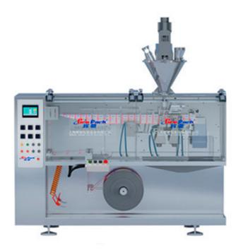
HC-110L horizontal packaging machine is an ideal bag packaging equipment that meets the requirements of high-quality packaging and smaller bags. The packaging speed is fast, and it can realize three-side sealing and four-side sealing bags; Packaging needs for various materials such as body and solid objects; roll film forming is used to reduce packaging costs.
