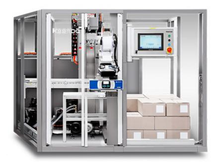
PT10 is a modular automatic robot palletizer that can be installed in compact area and it is applicable to variety of pallet patterns through HMI.
