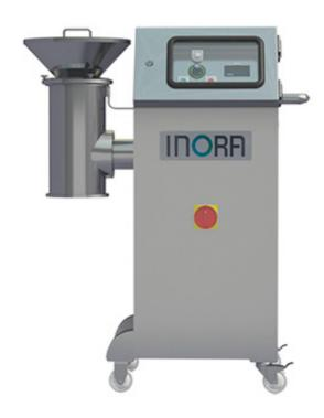
Cone milling is one of the most common methods of milling in the pharmaceutical, food, chemical and associated industries. They are typically used for size reduction and agglomeration or dumping of powders and granules.
