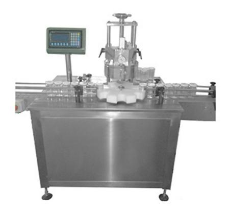
Completely into the bottle – vacuum – cap – out of the bottle. It is the ideal choice for food – beverage – canned/pharmaceutical industries.
