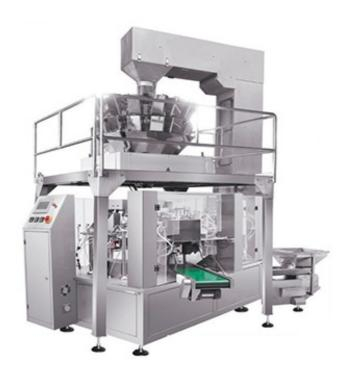
This line mainly installs rotary packing machine, combination weigher and Z-Conveyor, suitable for packing all kinds of grains and solids, such as candy, nuts, raisins, peanuts, melon seeds, potato chips, chocolate, biscuits and so on.
