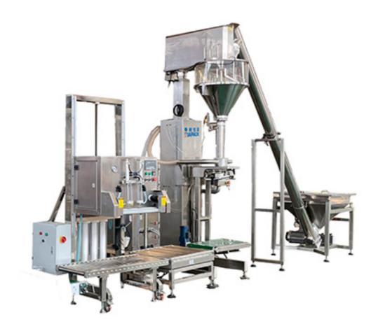
This model is designed mainly for the fine powder which easily to spout dust and high-accuracy packing requirement. Based on the feedback sign given by below weight sensor, this machine do measuring, two-filling (Fast filling and accuracy filling), and up-down work etc. It is specially suitable for filling additives, carbon powder, dry powder of fire extinguisher, and other fine powder which needs high packing accuracy.
