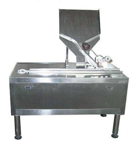
This machine is applied to the needle ampoule bottle printing, applied ampoule: 1-2 ml, 5-10 ml and 20 ml. The work table of the machine is made of 304# stainless steel; washing is easy, meet the GMP standard.
