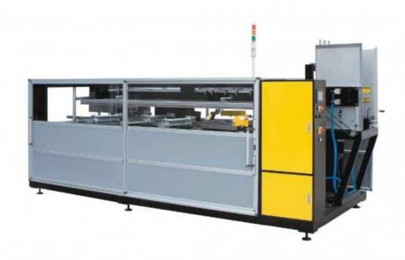
Case equipment is used to erect, pack, seal, or unpack cases of products. In most instances, case equipment is used to form cardboard boxes; however, corrugated materials and plastics formers are also available. Types of case equipment include case erectors, case cartoners, carton packers, carton sealers, and unpackers.
