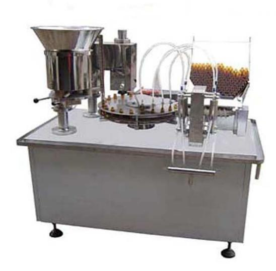
This machine is the main filling equipment of the oral liquor assembly line, which is mainly applied in the filling, lading, sealing of the 5-30ml EPOL (or aluminum plastic combined lid) straight tube bottle and realize reliable bottle transportation by screw, track the local filling process, and is not easy to produce foam; It transports the lid by electromagnetic vibration with high lading rate. This machine is advanced in its combined filling-sealing operation with the compact structure.
