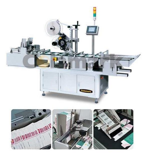
A751 is specifically designed for automatic feeding and labeling on flat items such as unfolded cartons, leaflets, cards and tags etc. Specially designed feeder handles various size and thickness of items smoothly. Suction assisted conveyor ensures stable transport of light and thin items and ensures precise label registration.
