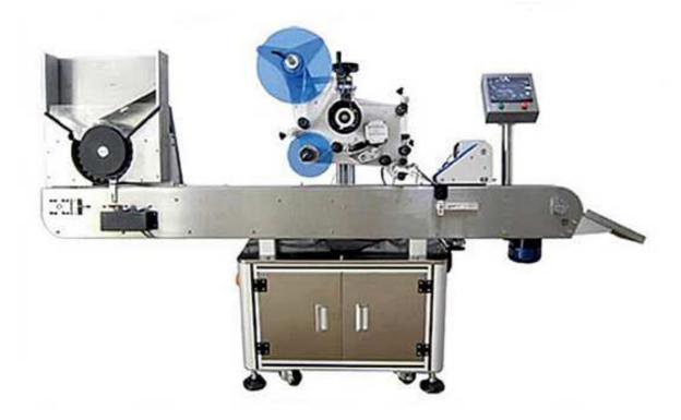
It adopt horizontal type transmission, horizontal type labeling, more stable, more precise and improve working efficiency It's applied to label the self-adhesive label on various small cylinder products, as small bottle, ampoule, lipstick, pen etc. This machine is widely used in electrical, pharmacy, foodstuff, and beverage, cosmetic and chemical etc industries.
