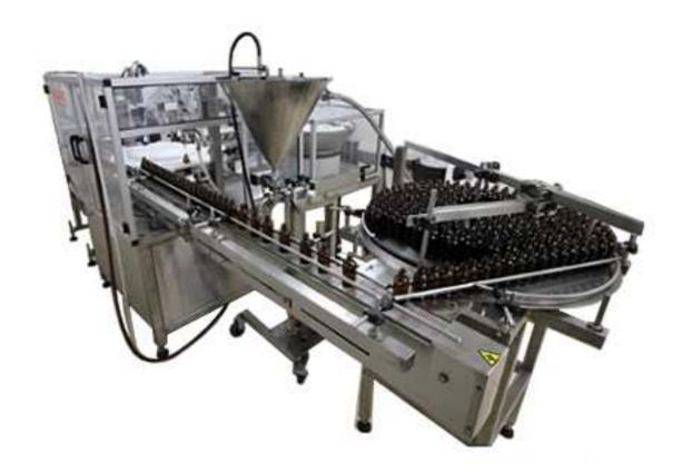
Impac Engineering Ltd. Developed the TORNADO series to address the necessity of filling liquids in small bottles with pipette.
