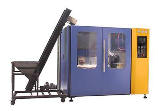
This two-step manually perform inserted full-auto bottle blower is applicable for blowing the carbonic acid beverage bottle, mineral spring water bottle, farm chemical bottle, oil bottle, medical, hot-filled bottle in any shapes and made of PET, PC, PP or PE raw material.
