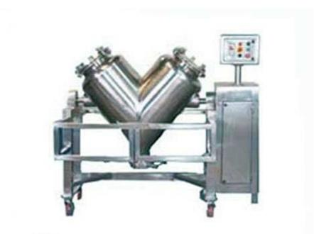
The rotating shell V-Type blenders are used only for dry mixes and have no packing glands (seals) around shafts entering the chamber to cause potential problems. Modifications such as the addition of baffles to increase mixing shear have been made to these types of blenders.
