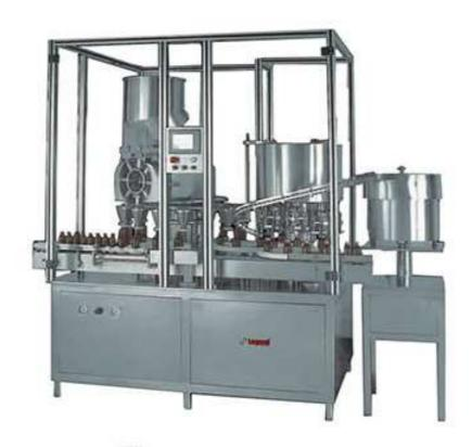
Legend Automatic High Speed 16 Head Rotary Dry Syrup Powder Filling Machine Model is suitable for Glass, Plastic, PET, HDPE, and LDPE Bottles with maximum speed of 120 Bottles per minute depending on Powder Fill Volume, Type of Powder, Bottle Diameter and Bottle Neck Diameter.
