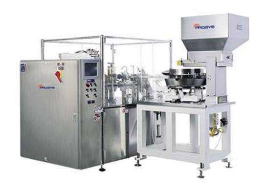
The RS12 with speeds to 60 has a 12 station dial which allows for additional post filling options perfect for cosmetic and pharmaceutical markets.
