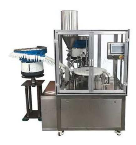
Filling and packaging of various syringes, boosters, injection tubes and the like in the fields of medicine, chemistry, biology and the like.
