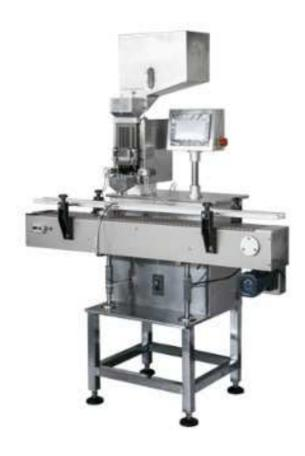
Capsule counter is designed to adopt unique multi-channel system with conveyor. The speed up to 30 bottles/minute based on 50 pieces/ bottle. The machine is only special for hard capsules.
