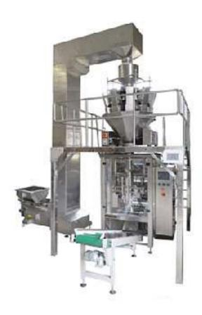
VFFS machine is a very popular machine for industries. It has a wide application for form fill seal. Such as granules, liquid, powder, jam, sauce, ketchup, etc. Variable package styles, pillow pouch, gusseted pouch, hand-hold pouch, fast speed makes it an excellent packaging machine. The maximum film width is 420mm. The packaging speed can be up to 80 bags per minute.
