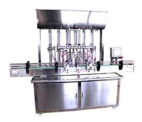
This series of liquid filling machine is suitable for filling different types of liquid products in daily chemical, food, grease, medicine, pesticide and other industries. The piston injection filling and three way one-way valve device has the advantages of high filling accuracy, convenient installation and debugging, simple cleaning and cleaning, and no leakage.
