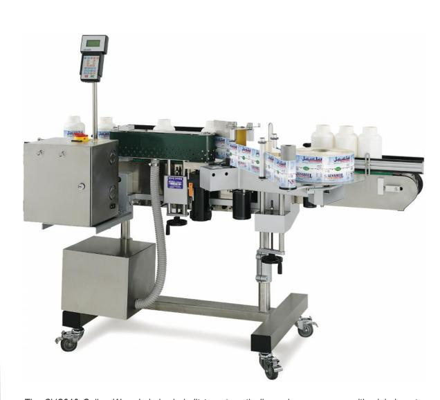
The CVC310 Gallon Wrap Labeler is built to automatically apply *pressure sensitive* labels onto large diameter round containers. The 310's extended wrap station includes a vacuum system for applying labels up to 17.5" in length and can be ordered with a 10" wide conveyor. The 310 is an ideal machine for contract packagers and manufacturers serving the nutraceutical, food, chemical, personal care, and household product markets.
