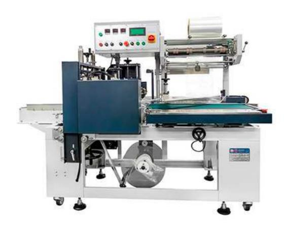
Auto Side Sealing Machine, standard model USA-005R can adjust its packaging height basing on product to have strong seal & nice look. Sealing safety sensor prevent the product from damaging by cutting & protect sealing knife without injury.
