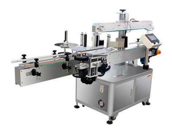
YG-620GS single-side bottle labeling machine for square bottles or flat shape of things off the side of the bottle label can be installed independent of plastic bodies, specialized cosmetics industry for automatic labeling and other irregular shape of the object; roll can be installed standard devices.
