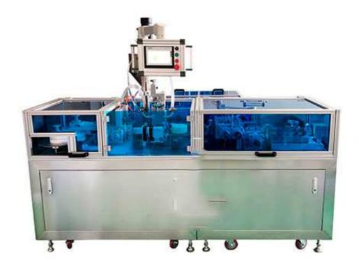
SP-2 type suppository filling automatic production line has a stable and efficient preheating mold, heated mold, molding, belting, canned, frozen, sealing bolt all production processes such as complete system process, grain production capacity of 3000-4000 / hour.
