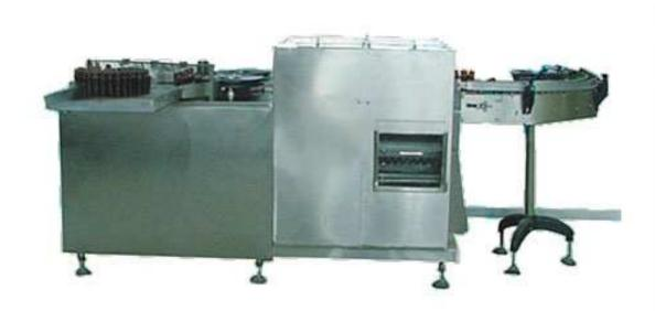
The drum ultrasonic washing machine is a kind of cleaning equipment for penicillin bottles and oral liquid bottles. Rotary drum structure is designed for it, and bottles need to be cleaned several times in this drum ultrasonic washing machine. First, they are washed by ultrasonic waves. Then they will be cleaned by running water, distilled water and purified compressed air in turn.
