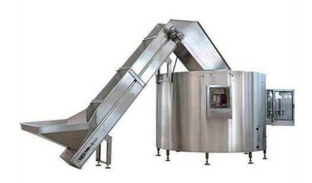
This Full Automatic Bottle Unscrambler is used in ordering disordered polyester bottles. The disordered bottles are carried into the storing bottle section of the ordering bottle machine. With the help of the pushing force of the rotating disk, the bottles enter their position. With the function of the turning bottle device and the air-flow, the bottles are ordered into bottle mouth-up-position and are carried into the next process with the air-transfer type conveying bottle system.
