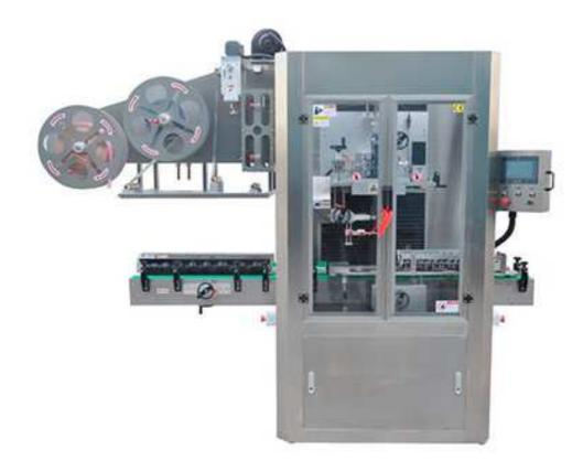
Sleeve labeling machine, also called sleeves labels applicator or sleeves labels inserting machine, which cut sleeves piece by piece and insert the sleeves to bottles, and then shrink the sleeves labels by steam shrinking tunnel or electrical heating tunnel to bottles tightly. The sleeves can label bottles' body or seal bottles' caps and necks.
