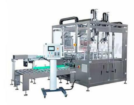
The machine is automatic finishing massive items and put them into the cartons with manipulator. It is a high efficiency and energy saving which can replace artificial packing.
